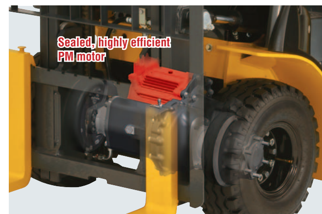
Sealed, highly efficient PM motor
